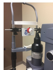
Figure 1. Example of laser simulation setup with the SimuEYE 400 lamp holder and SimuEYE LPI model eye.
